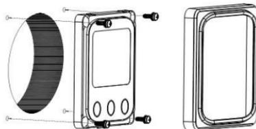
**Step1:** Locate and drill screw holes based on the installation size of the surface.
