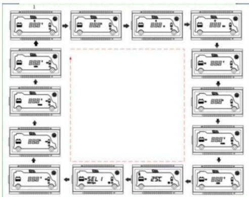
Echo Loop: PV voltage —PV current —PV power—Battery power—BATT1 voltage—
