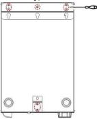
Step2: Mark the installation position with the mounting plate 1. The distance between the two mounting holes is 300mm.
